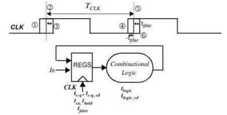
Figure: Circuit for studying the impact of jitter on performance.
