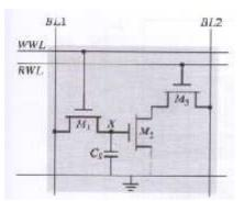
Figure: Three transistor dynamic memory cell
