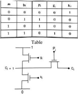
Figure – switch level circuit
