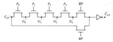
Figure: Manchester carry-chain implementation of bypass adder
