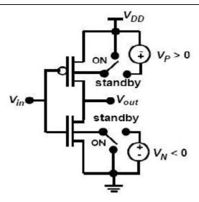
Figure: Variable Body Biasing
