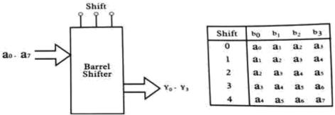
Figure: 8 X 4 barrel shifter
