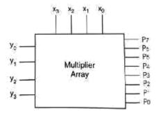
Figure: General block diagram of multiplier
