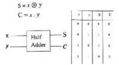
Figure: Half adder and Truth table
