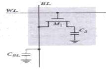
Figure: One transistor DRAM
