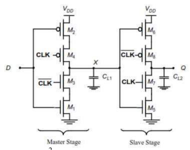
Figure 3.16  $C^2$ MOS master-slave positive edge-triggered register.
