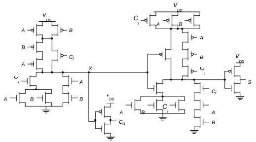
Figure: Complimentary Static CMOS Full Adder
