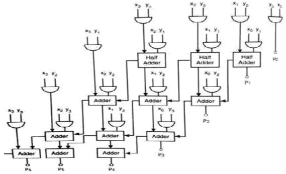
Figure: 4 x 4 array multiplier
