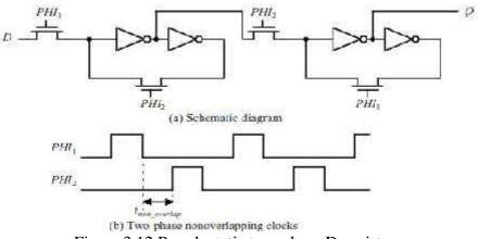
Figure 3.12 Pseudostatic two-phase D register.
