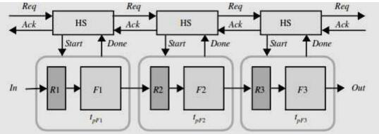
Figure: Self-timed, pipelined datapath.
