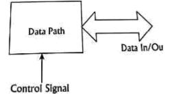
• Data path block consists of arithmetic operation, logical operation, shift operation and temporary storage of operands.
