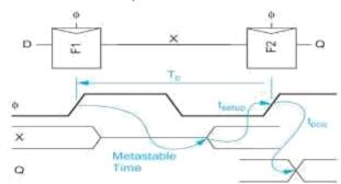
Figure: Simple Synchronizer
