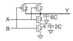
Figure: 2 -input NAND gate Schematic Y=A.B
