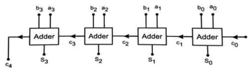
Figure: Ripple carry adder
