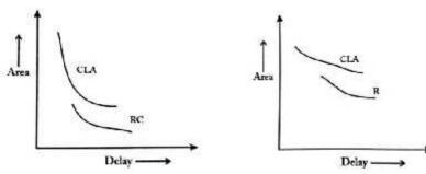
Figure: Area Vs Delay for 8 bit adder
