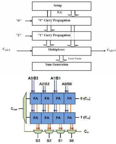
Figure: Building blocks of a carry-select adder
