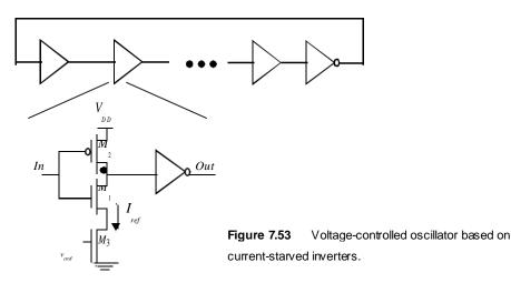
In this modified inverter circuit, the maximal discharge current of the inverter is lim-ited by adding an extra series device. Note that the low-to-high transition on the inverter can also be controlled by adding a PMOS device in series with  $M_2$ .
