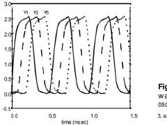
Figure 7.52 Simulated waveforms of five-stage ring oscillator. The outputs of stages 1, 3, and 5 are shown.
