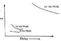
Figure: Area Vs Delay for all multiplier
