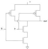
And here is a stick diagram for the two-input NAND:
