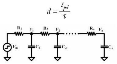
Figure: RC delay equivalent for series of transistors
