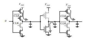
Figure 3.25 Potential race condition during (0-0) overlap in C<sup>2</sup>MOS-based design.
