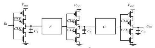
Figure 3.24 Pipe lined datapath using C<sup>2</sup>MOS latches
