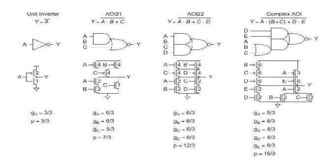
Figure: Logical efforts and parasitic delays of AOI gates
