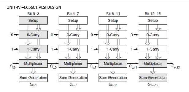
Figure: general structure of 16 bit adder
