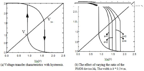
Figure 7.49 Schmitttrigger simulations.
