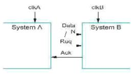
Figure: Communication between asynchronous systems
