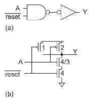
Figure: Resettable buffer optimized for data input
