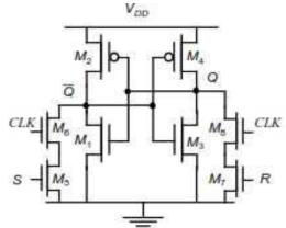
Figure 3.5 CMOS clocked SR flip-flop
