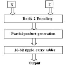
Figure: Block diagram of Booth multiplier
