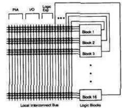
Figure: Altera Max 5000 Routing Architecture
