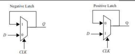
Figure 3.6 Negative and positive latches based on multiplexers.
