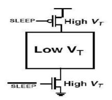
**Figure10: Circuit Design with Sleep Transistors**
