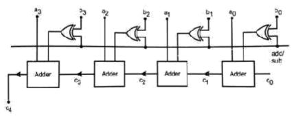
Figure: 4-bit adder/subtractor circuit
