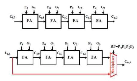
Figure: (a) Carry propagation (b) Adding a bypass
