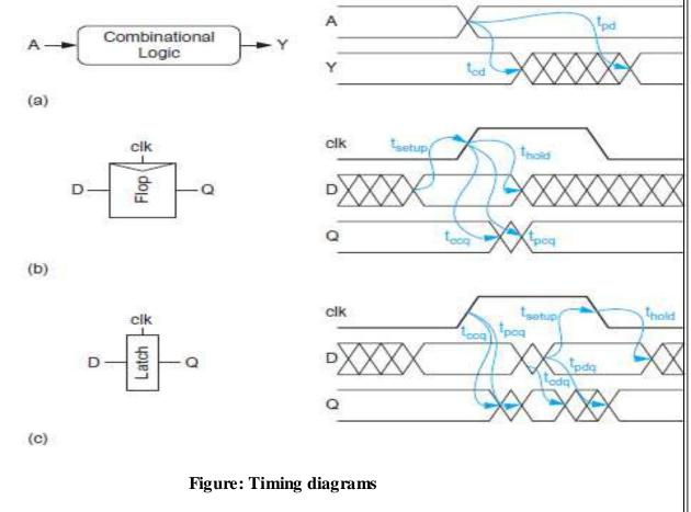
• The output begins to change after a clock-to-contamination delay  $\{t_{ccq}\}$  and completely settles after clock to-Q propagation delay  $\{t_{pcq}\}$ .
