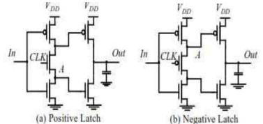
Figure 3.20 Simplified TSPC latch (also called split-output).
