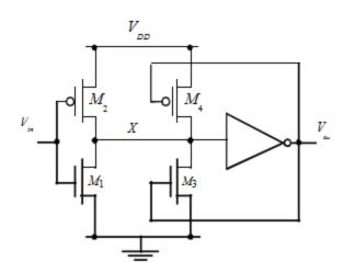
Figure 7.48 CMOS Schmitt trigger.
