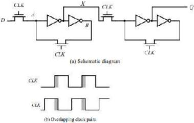
Figure 3.11 Master-slave register based on NMOS-only pass transistors.
