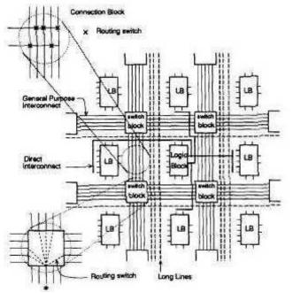
Figure: Xilinix Routing Architecture
