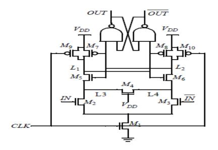
Positive edge-triggered register based on sense-amplifier
