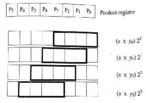
• A practical implementation is based on the sequence. The product is obtained by successive addition and shift right operations
